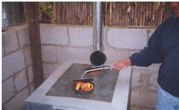
**Portable plancha stove manufactured by Manuel Tay in operation, with two pot holes and an edge.
