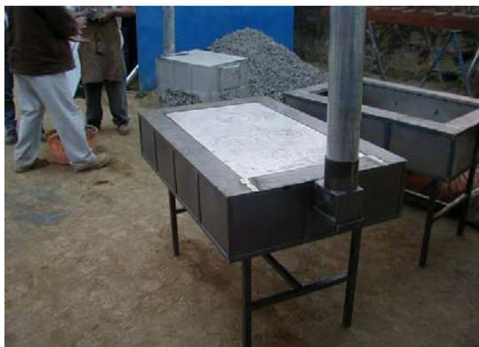
**Portable plancha stoves manufactured by Taller San Mateo, including small model at the back without protective edge.
