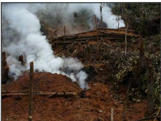
Traditional charcoal kilns in Madagascar, with nearly 2/3 of energy losses through the smoke
