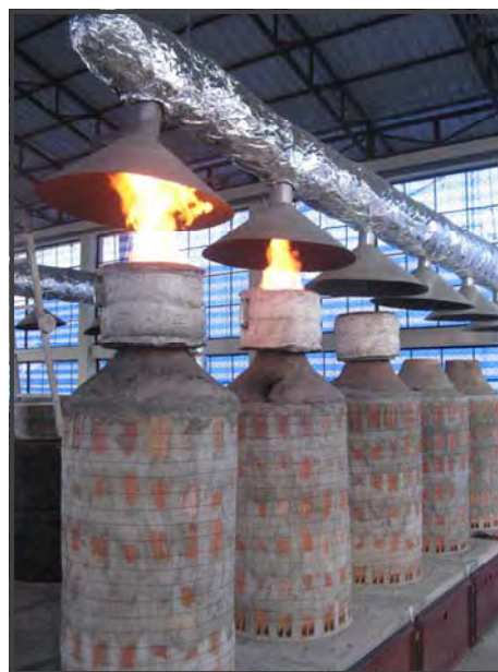
The natural draft T-LUD pyrolyser
