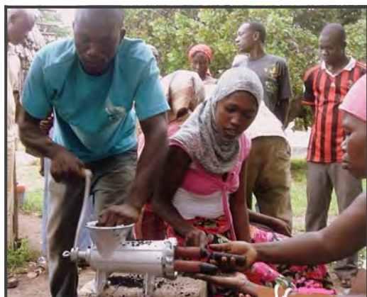
A team of 3 operating the manual extruder (one cranking, one feeding and one collecting briquettes)
