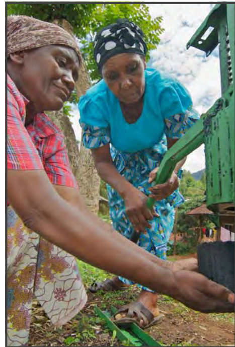
Extracting a briquette from the Ratchet Press, Lushoto Tanzania
