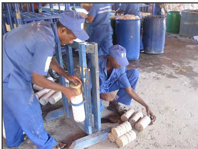
Final step in the briquette production process — factory employees releasing briquettes from their mold to dry in the sun
