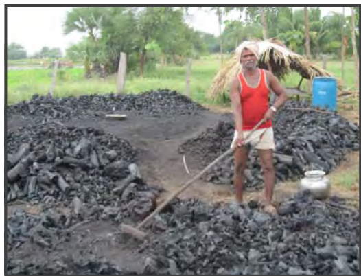
A charcoal producer harvesting the charcoal carefully (involves quenching the burning charcoal pieces with water)
