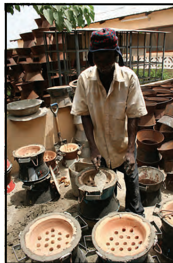
Toyola employee assembling stove bodies and liners
