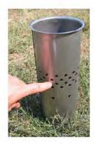
The Fire Grate Keep the top of the fuel below the triple-line of holes as shown in the photo. When burning dung, start a small wood fire first then add dung.
