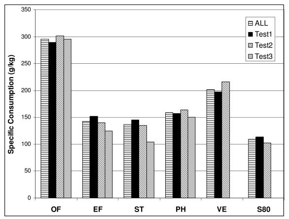
Figure 11. Specific consumption for each test number for the six stoves. The average of all tests is shown as well for each stove.
