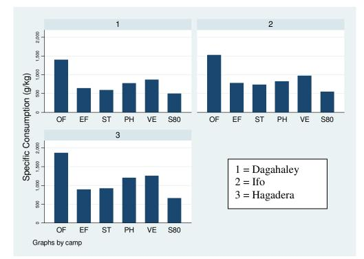
Figure 3. Average specific consumption (g/kg) for each stove type in each of the three camps of the Dadaab complex.
