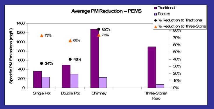
The non-chimney stoves reduced total PM by 34%-40% compared to traditional, and about 70% compared to the three-stone. The rocket chimney stove released 82% less PM out the chimney than cement chimney stove with poor draft.
