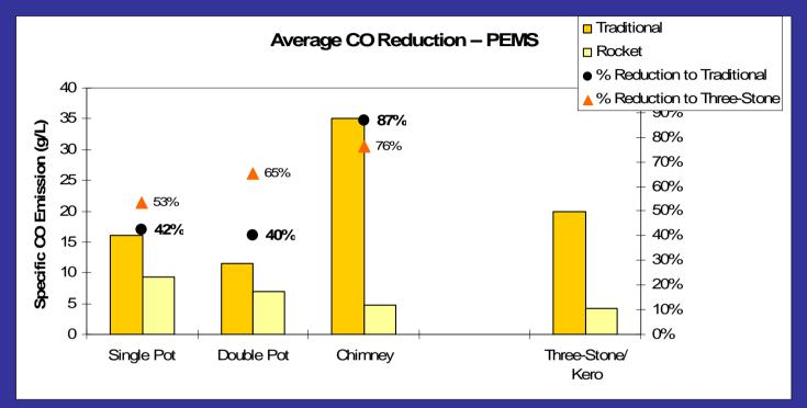
The rockets reduced CO by about 40% vs. traditional and 53-60% compared to the threestone. Similar to the PM results, insufficient draft resulted in high levels of CO from the traditional chimney stove.
