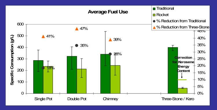
The rocket stoves saved between 18 and 35% of the fuel compared to the traditional stoves. When compared to the three-stone fire, the rockets saved about 40%.
